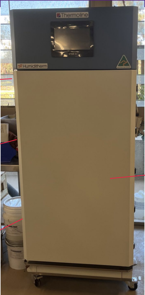
TEC carbonation chamber
